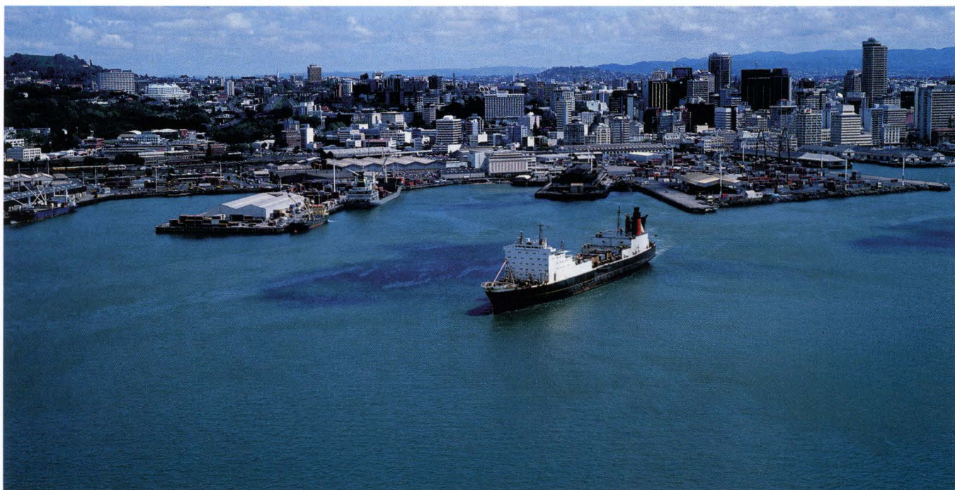
Container facilities continue to expand at Auckland. Bledisloe Wharf to the right has swallowed the old Kings Wharf; Bledisloe has ro-ro facilities and one container crane, and container storage creeps westwards along the north side of Quay Street. Ferguson Wharf, the main container wharf, with four cranes, is out of the picture left, to the east. (Ports of Auckland).
