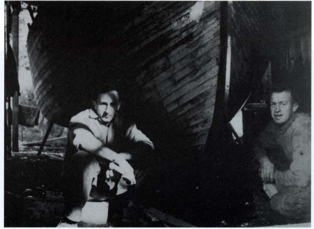
Ernie and Ted (right) beside the strip-planked hull of the DOLPHIN, 1948. They claim they built half each and that on completion one side was "four inches" longer than the other! (Ted Torkington)
